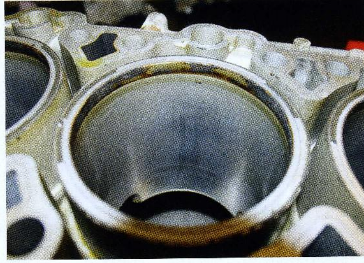
Clockwise from top left: Badly scored piston after prolonged cylinder contact and overheating. Replacement Hartech Nikasil-coated liner with closed deck top awaiting assembly in machined-out crankcase. A polished cylinder liner is acceptable at this stage. Bad cylinder scoring on the thrust face
