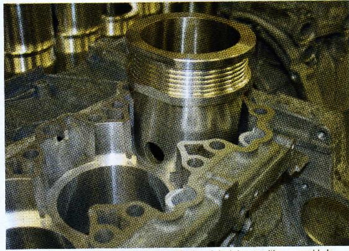
Clockwise from top left: Badly scored piston after prolonged cylinder contact and overheating. Replacement Hartech Nikasil-coated liner with closed deck top awaiting assembly in machined-out crankcase. A polished cylinder liner is acceptable at this stage. Bad cylinder scoring on the thrust face
